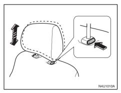
Push in the release button and press downward on the head restraint in order to adjust the position downward.
